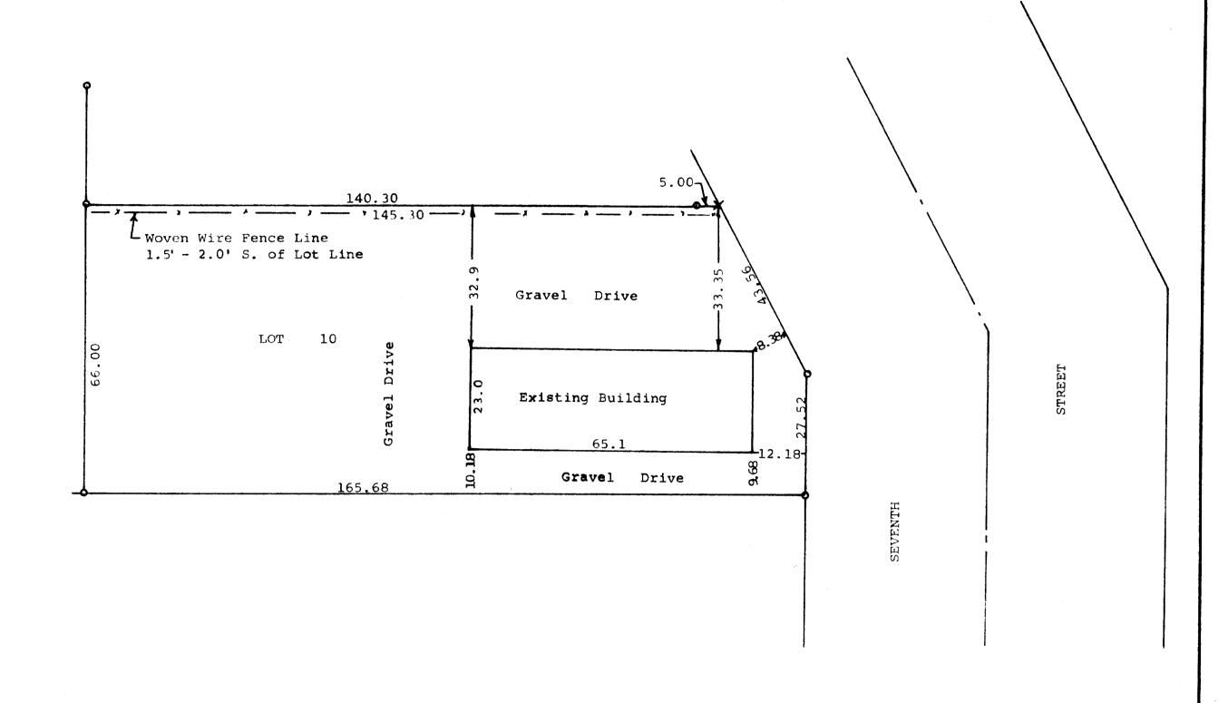
Scale - 1" = 20'• = Iron Pipe x = Cross in Concrete
